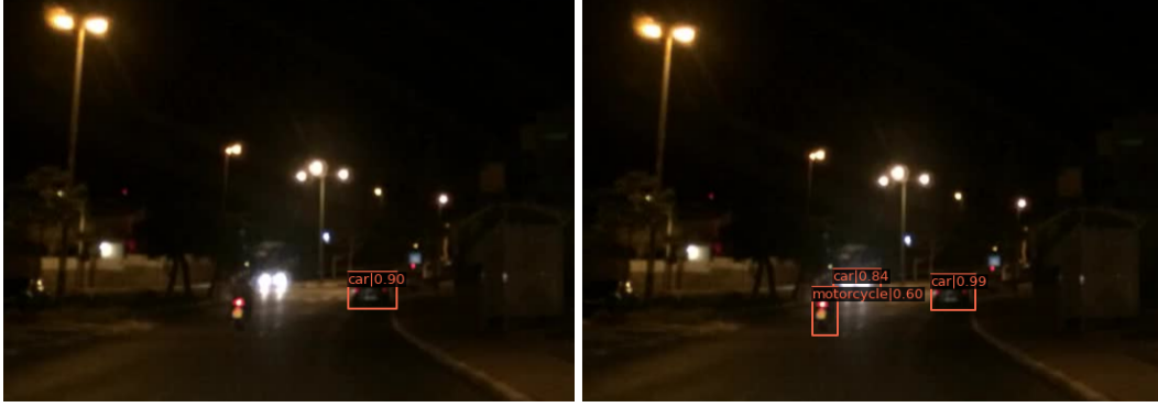
Figure 9: A false negative motorcycle at night on the road (left) fixed to a true positive detection (right) using TALISMAN.
